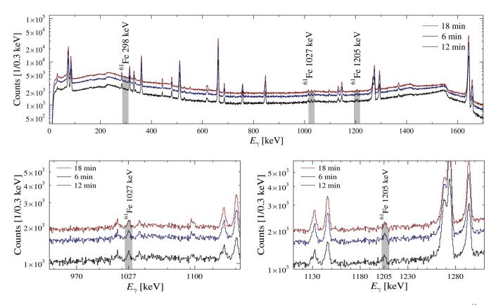
FIG. 6. (Color online) The  $\gamma$ -ray spectrum of the activation without cadmium shielding measured for one, two, and three half-lives of <sup>61</sup>Fe, respectively. The upper panel provides an overview, and the lower panels show a zoom into the regions of the <sup>61</sup>Fe lines at 1027 and 1205 keV. The background stems from the activation of the contaminants of the <sup>60</sup>Fe sample.
