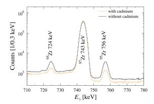
FIG. 5. (Color online) The  $\gamma$ -ray spectra of the Zr monitor foils used for the neutron fluence analysis normalized for different measuring times. Due to the smaller capture cross section of  ${}^{96}$ Zr in the thermal energy regime, the cadmium shielding affects the  ${}^{97}$ Zr signature to a much lower degree than that of  ${}^{95}$ Zr.
