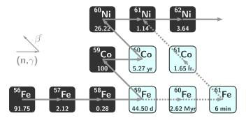
FIG. 1. (Color online) The *s*-process reaction path between Fe and Ni. The isotope <sup>60</sup>Fe is produced via a sequence of  $(n, \gamma)$  reactions starting at the stable iron isotopes. Because of the short half-life of <sup>59</sup>Fe ( $t_{1/2} \approx 45$  d), the production of <sup>60</sup>Fe depends critically on the stellar neutron density.
