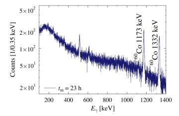
FIG. 4. (Color online)  $\gamma$ -ray spectrum for the determination of the <sup>60</sup>Co activity taken 34 months after purification of the sample. The measurement time was  $t_m = 23$  h.
