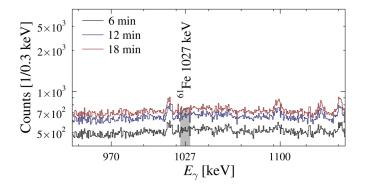
FIG. 7. (Color online) A detailed view into the region around 1027 keV of the  $\gamma$ -ray spectrum after activation with the cadmium shielding, illustrating the absence of <sup>61</sup>Fe lines. Therefore, only an upper limit can be deduced from the data.
