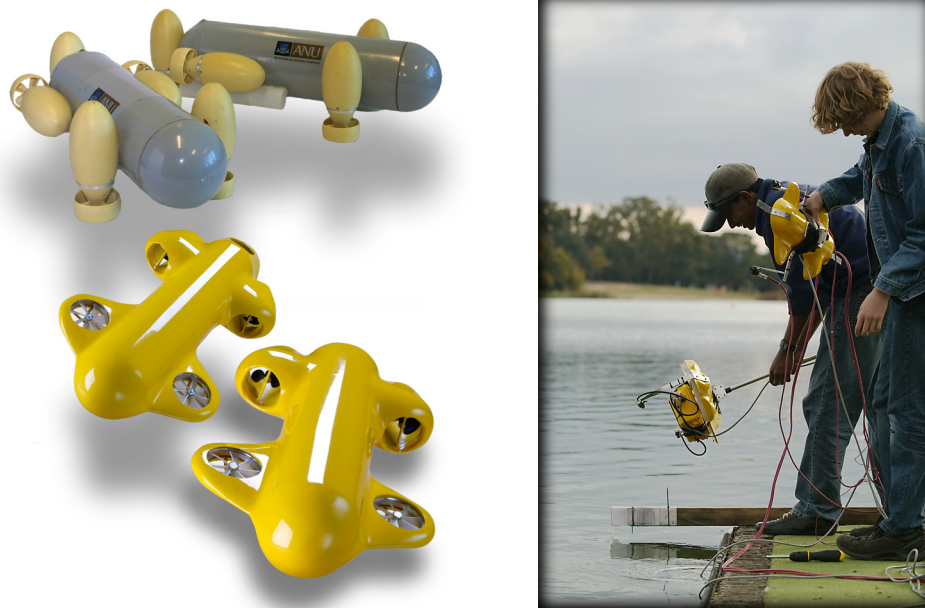
Figure 1.1: Serafina Mk I AUVs [top left], prototype Serafina Mk II AUVs [bottom left] and the author and Jan Zimmer setting up localisation experiments using mock-up hulls [right].
