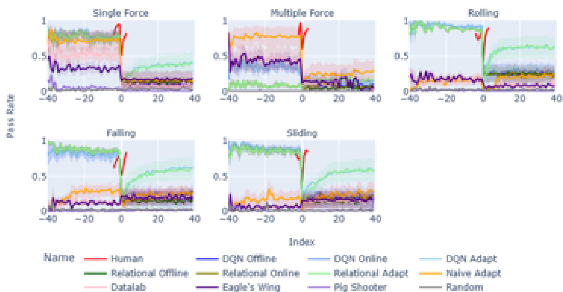
Figure 5.9: The pass rate of the agents per scenario. x-axis represents the index of the task in trials. Indexes -40 to -1 represent normal tasks and 0 to 40 represent novel tasks. The y-axis shows the pass rate averaged across all trials relevant to the respective scenario. DQN Adapt and Relational Adapt are the agents with NAPPING, which is discussed in Chapter 6.
