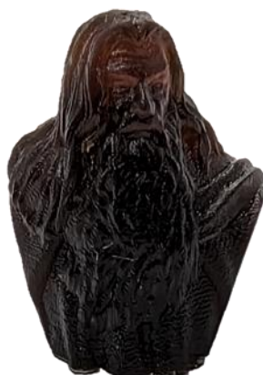
Figure 4.4. The 3D printed Gandalf figurine using the PEGDA 700/water (8/1, w/w) in the presence of ellagic acid/Iod (0.3%/2%, wt) and 100 mM NaOH. (9 × 10 × 13 mm, L × W × H; layered exposure time: 10 s)
