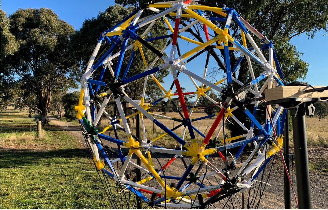
Figure 6.2: The setup for single propeller noise measurement. The propeller is placed at the center of microphone array, and 32 microphones are nearly uniformed arranged over the lower hemisphere.
