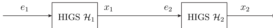
Figure 9.4: A cascade of the HIGS \mathcal{H}_1 and the HIGS \mathcal{H}_2 . The output x_1 of \mathcal{H}_1 is fed into \mathcal{H}_2 as its input e_2 .
