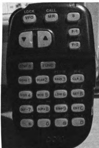
Figure 13 Microphone on ICOM IC-2100 VHF transceiver
