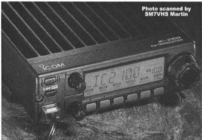
Figure 11 ICOM IC-2100 VHF transceiver
