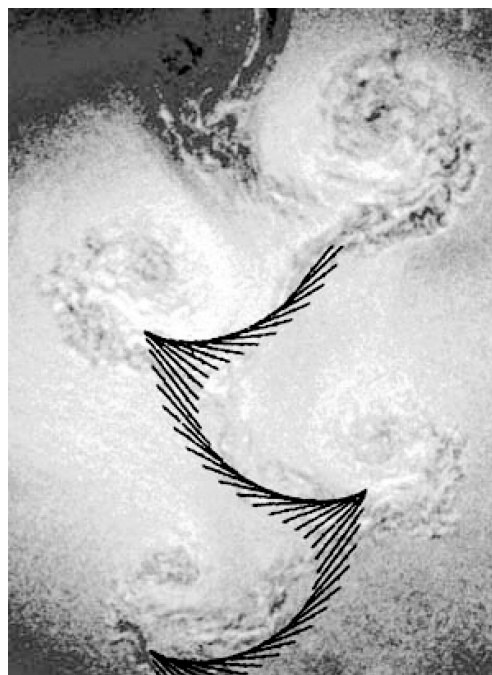
Figure 1. The path of a sinking strip superimposed onto an image of the vortices it creates, taken from Belmonte & Moses (1999). This motion demonstrates the effect shape can play in controlling the vertical, horizontal and rotational motion of a sinking body.
