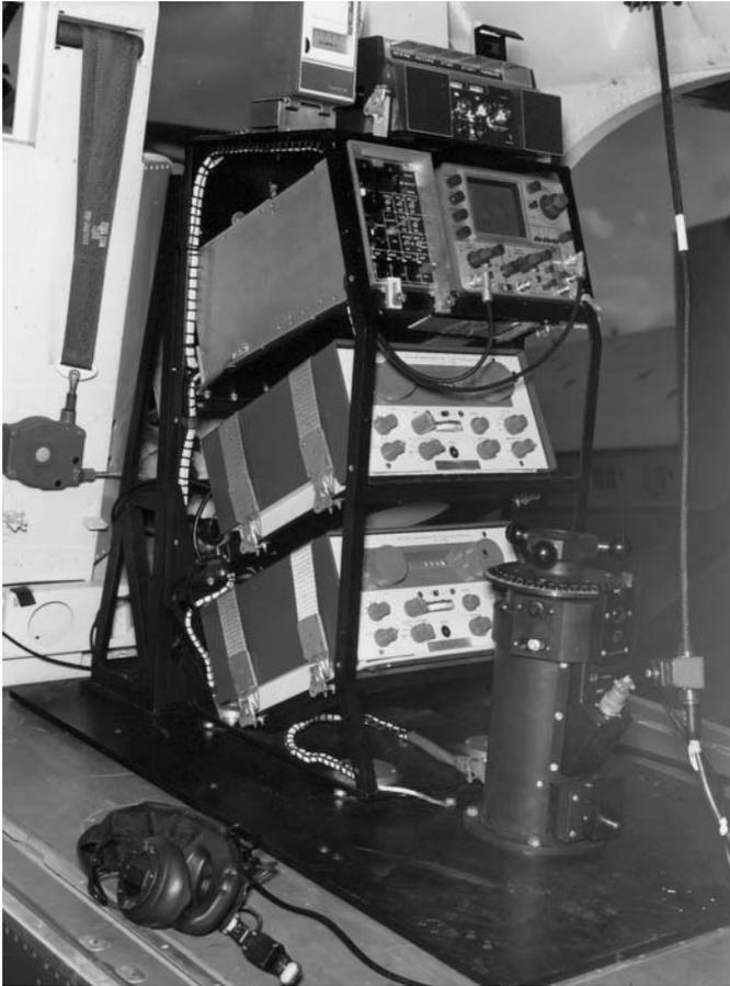
*Plate 4: ARDF Console installed in Pilatus Porter aircraft.*
