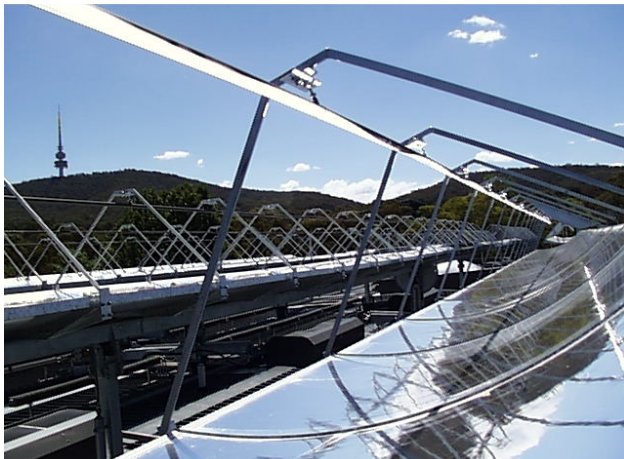
Figure 3 Mirror panels focus light onto a test receiver
