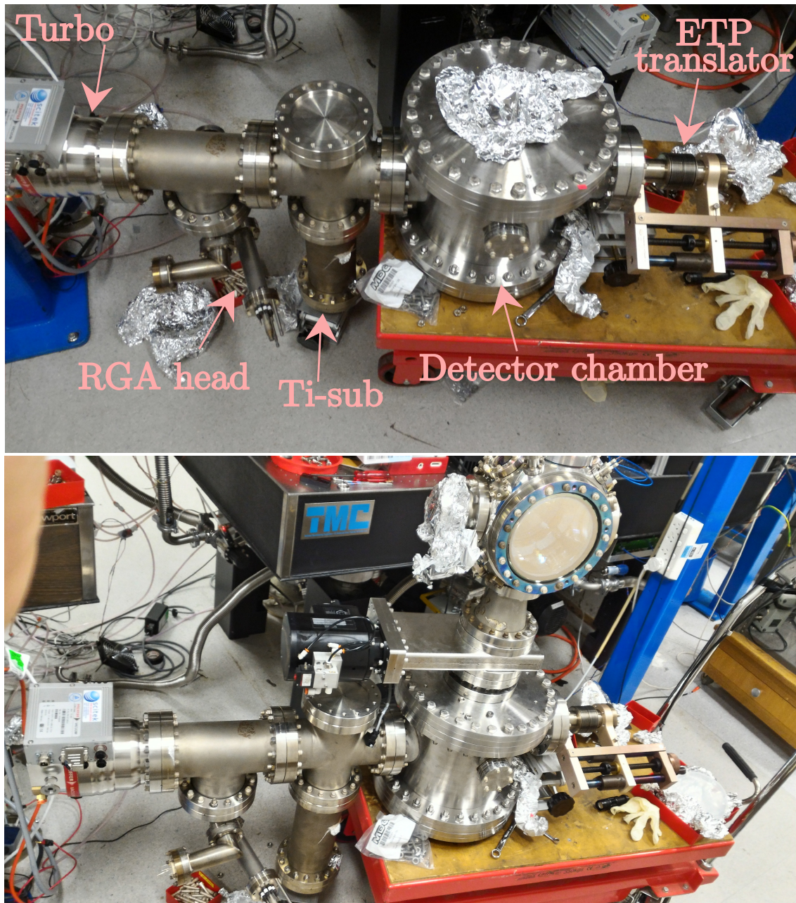
Figure A.3: Top: The leviathan-like underbelly of the science chamber resting after assembly on the mobile pallet jack and a smaller hand jack to support the TiSub. Bottom: The science chamber was re-mounted with an intermediate gate valve and then wheeled into place. The assembly was stabilized on the blank flange at the bottom of the 24"-diameter detector chamber, and by being really heavy.
