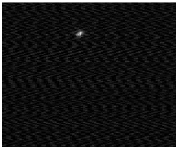
Figure 2. Controller prototype on-sky image of HR4458 M=6 star-system with evident pattern noise (April 2019)
