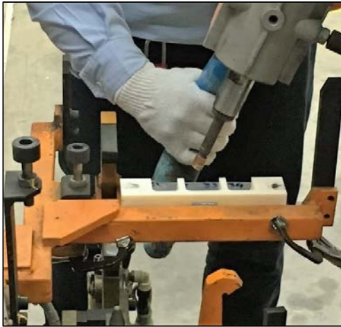
Figure 3: Misalignment of weld gun to produce poor quality welds
