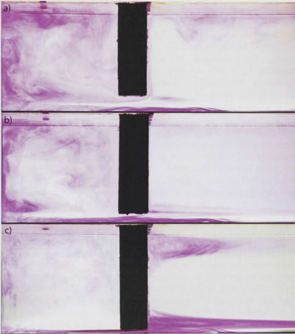
Figure 3.7: Photos of experiments with an imposed flux and a flat sill with R_D = (a) 0.15, (b) 0.1 and (c) 0.05. Only the left-hand (heated) half of the tank is shown. Dye tracer was added as in figure 3.6.
