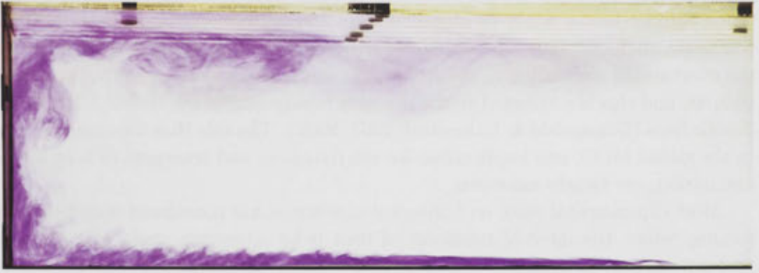
Figure 1.2: The ‘polar’ end of a laboratory experiment of horizontal convection driven by thermal boundary conditions of a piecewise uniform temperature difference at the base of the tank. This laboratory experiment is inverted relative to the oceans.
