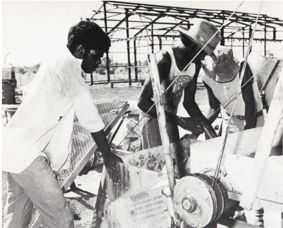
Plate VI (above) Smiler Gordon, Joseph Green and Brian Hargraves operate a brick making machine at Hooker Creek.
