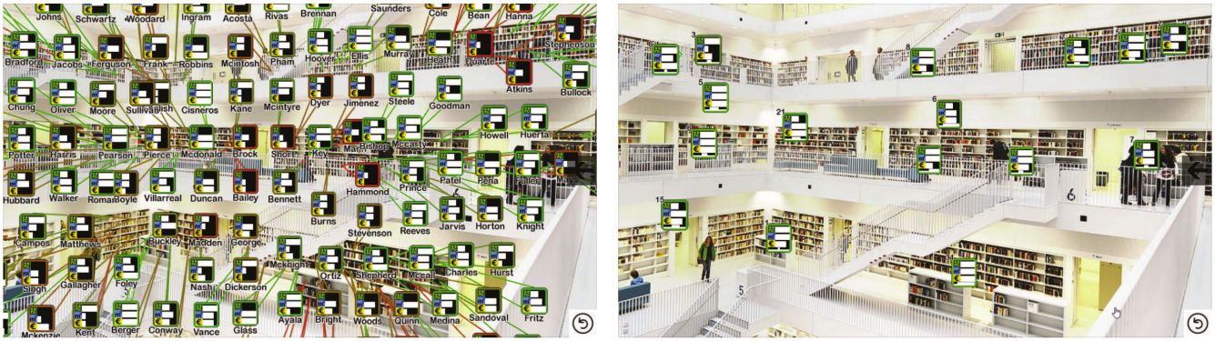
Figure 2: AR augments human perception with additional context-based information. Unchecked augmentation can quickly lead to clutter distracting users on-the-move causing safety issues. Adaptive visualization, as shown here, adjust information density and presentation style to balance the information in the user’s view [80]. How can adaptive visualizations help users with AR on-the-move?
