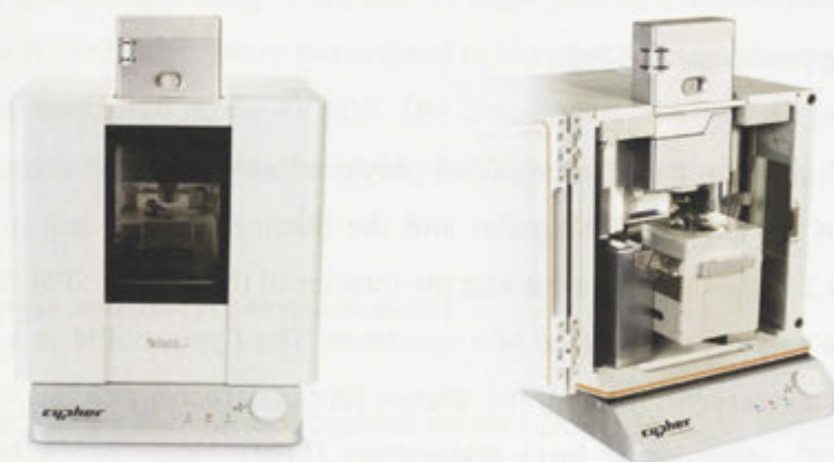
Figure 2.7 Photographs of the exterior (left) and the interior (right) of the Cypher scanning probe microscope.
