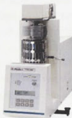
Figure 2.4 Photo of the Shimadzu 50 TGA instrument.
