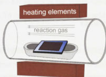
Figure 2.3 Schematic diagram of a typical horizontal furnace with heating elements and a heating tube containing an alumina crucible and the sample.
