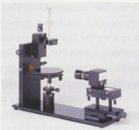
Figure 2.6 Photo of the optical contact angle and surface tension meter (CAM 101).
