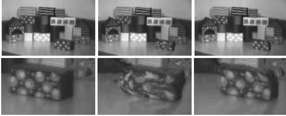
Fig. 7. A 540nm band (left) is sequentially registered from frame 6 to 1 using inter-band optical flow (center) and spatio-spectral image-based optical flow (right).
