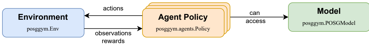
Figure 6.2: POSGGym’s high-level architecture. Agents interact with the environment by selecting actions according to their policy which has access to a model of the environment for planning.
