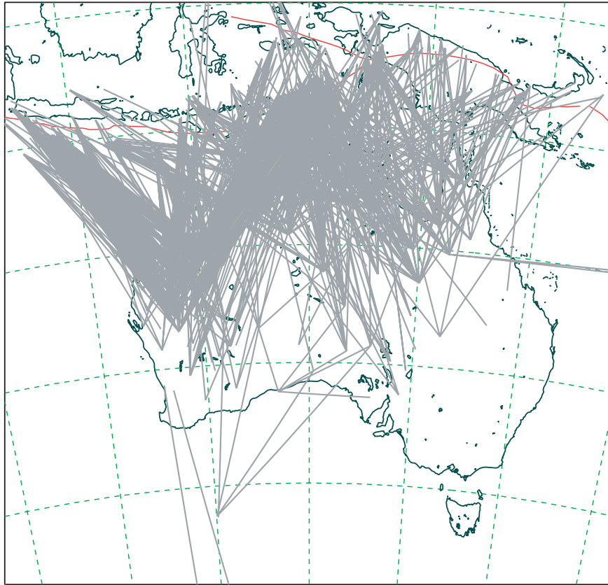
Figure 6. Paths with very small differential attenuation \delta t_{sp}^* < 0.2 determined from the spectral ratio of S and P waves. Most of these paths traverse the cratonic regions of Australia and display the characteristic long and high-frequency P and S coda displayed in earlier figures.
