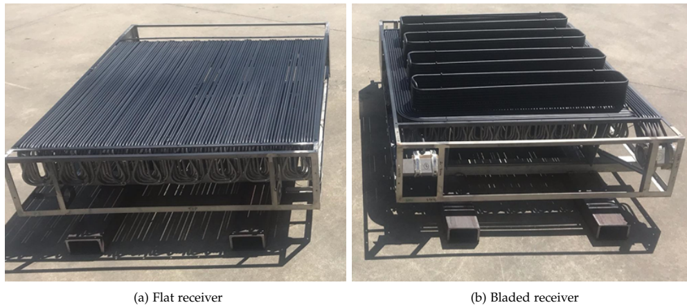
Fig. 4.22: Full pictures of (a) flat and (b) bladed receivers with Pyromark coating.
