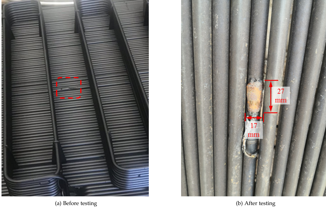
Fig. 5.11: The welding of the thermocouple on the receiver (a) before and (b) after on-sun testing. The surface appearance after on-sun testing (b) indicates a significant difference in surface emissivity from before testing (a) 4 .
