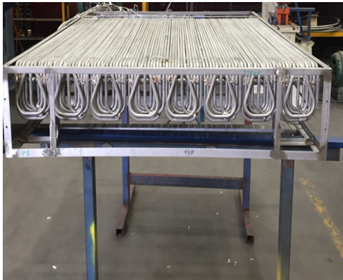
(a) The full picture of the bends from top of the receiver
