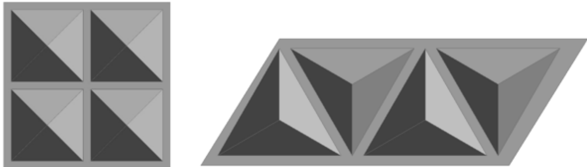
Figure 3.19 Geometry of the pyramidal (left) and tetrahedral (right) panel with gaps between protrusions.
