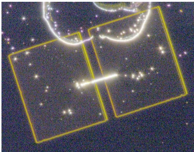
Fig. 4.7. Gold electrodes linked by a crystal of rotaxane 4.2 .
