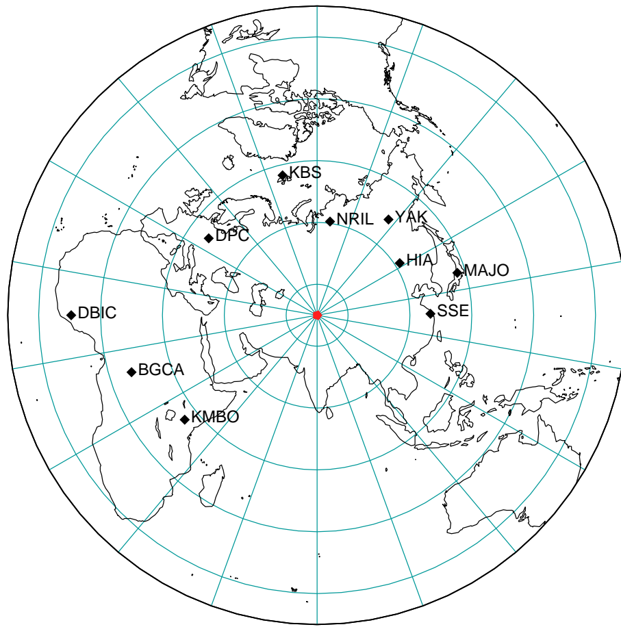
Fig. 5.6. Location of the 6 April 1997 southern Xinjiang event along with the station distribution used in the inversion.
