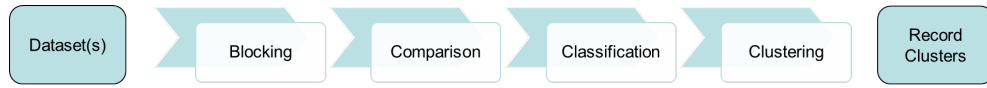
Figure 1.1: A general process of ER. One or more datasets after pre-processing (e.g. data cleaning) are used as input, and clusters of records referring to the same real-world entities are generated as output.
