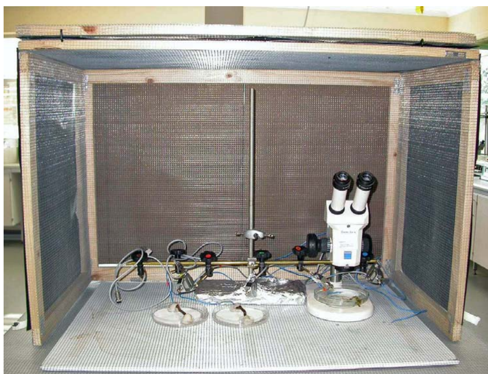
Figure 4. The faraday cage used for all EPG recordings; the access door was opened during the set up of the plant and insect electrodes, and closed during recordings to reduce the level of background electrical interference. The pictured set up contains the tissue culture plant system with the stereo microscope (right), and two excised root systems (left). The wire exterior of the faraday cage was covered with black cardboard to provide a dark environment for the radicicolae grape phylloxera.
