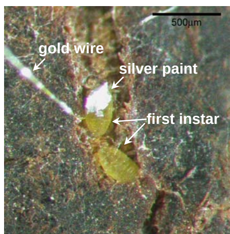
Figure 3. First instar grape phylloxera on an excised root piece in the active feeding position and connected to the insect electrode. The main features of the insect electrode are labelled with arrows, including the short section of 12.5 \mu\text{m} gold wire and the conductive silver paint. Scale bar 500 \mu\text{m} .
