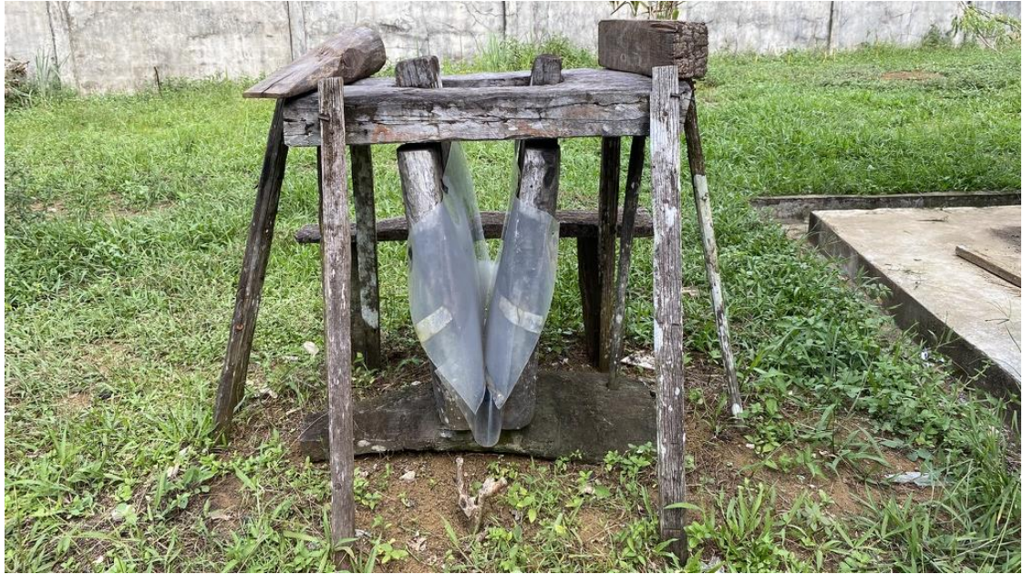
Figure 4.5 Apit , the traditional tengkawang oil extraction tool made from ironwood, which is no longer used and is currently displayed in the mini-factory.
