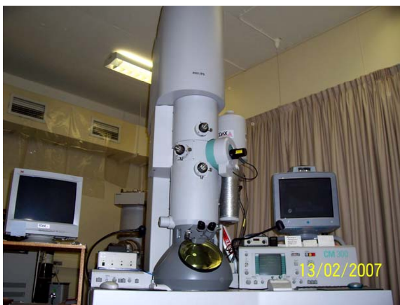
Fig 3.4: Geometrical optics representation of the TEM (a) BF imaging mode and (b) Diffraction mode. And the Philips CM 300 Transmission Electron Microscope.
