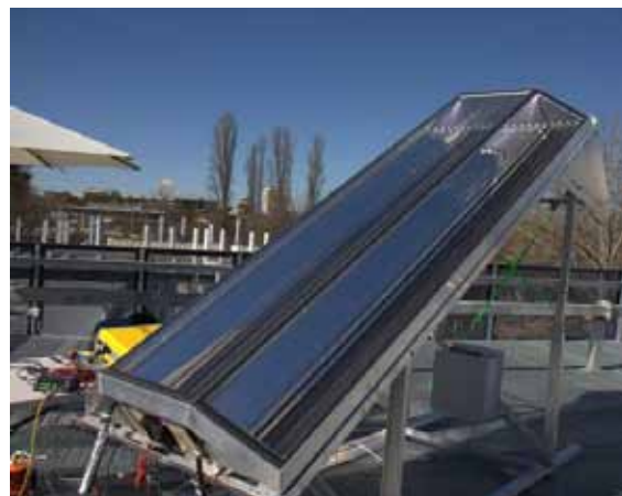
Figure 1: First prototype MCT system mounted and operating on the roof-top test platform at ANU.
