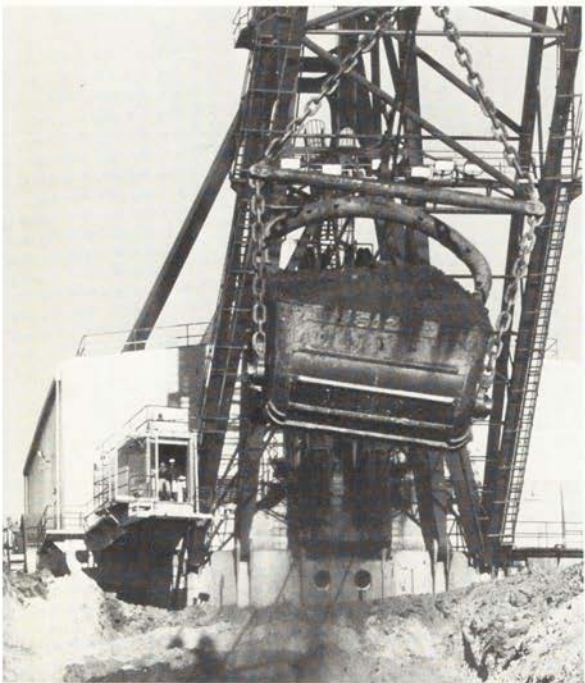
Above: A huge electrically powered walking dragline, Saraji Mine, Bowen Basin, Queensland.
