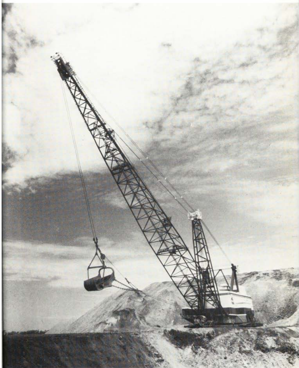
A walking dragline uncovering a coal seam, Goonyella mine, Bowen Basin, Queensland. By courtesy of Utah.
