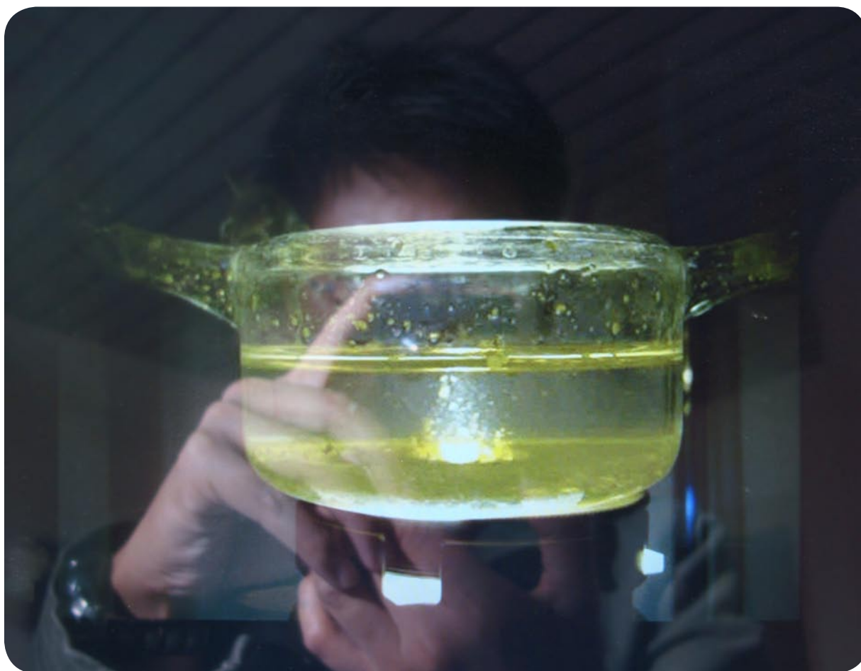
Zhiguo photographs the vigorous stream of oxygen bubbles rising from a silver orthophosphate solution when a bright light spot shines on it
