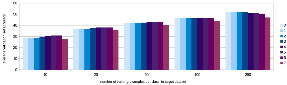
Figure 7.5: Number of frozen pretrained layers. The effect on performance of the number of pretrained layers of weights frozen during fine-tuning are shown across various target dataset sizes.
