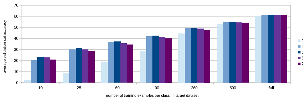
Figure 7.1: Number of layers transferred vs dataset size. Each bar represents the average accuracy over the validation set for a model fine-tuned on one size of target training dataset with a particular number of layers of pretrained weights transferred.
