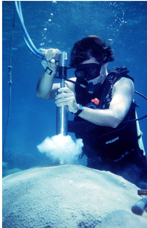
Figure 2.2 D. Whitford using core barrel to flush cuttings to prevent core barrel seizure.
