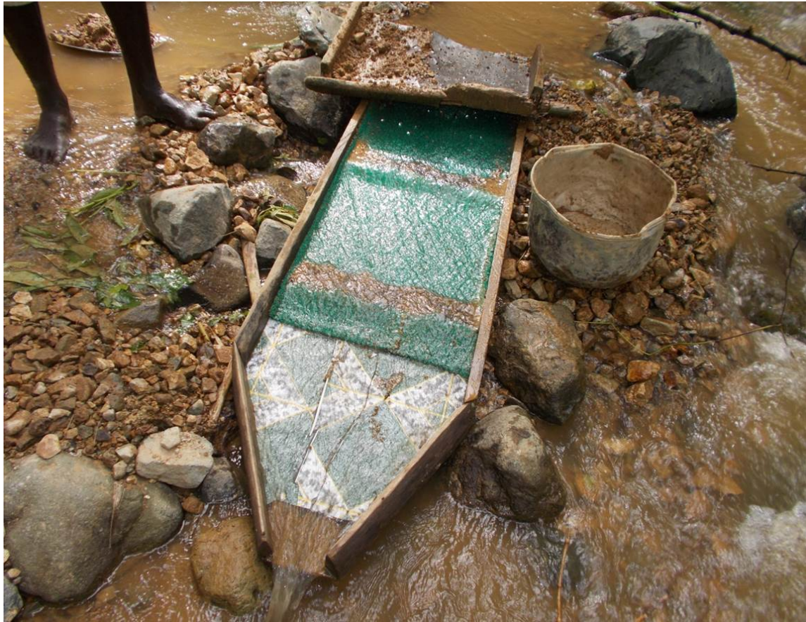
Sluice box made with scrap bush materials and carpet.
