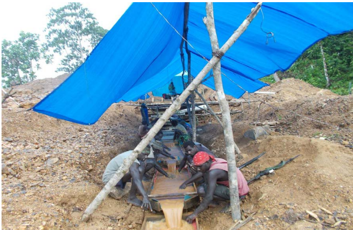
Sluicing method adapted from sago processing at Sinimi.
