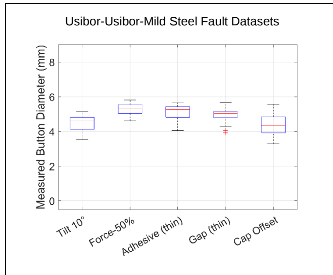
Figure 4-11: Usibor-Usibor-Mild fault dataset destructive testing summaries
