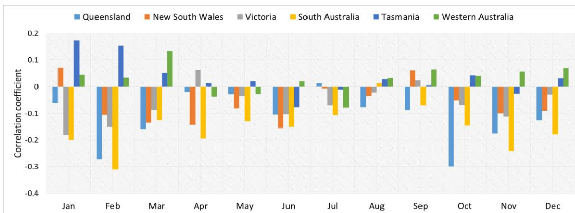
Figure 1-14 Correlations between solar and wind resources in each state/territory of Australia (except Northern Territory). Low correlation coefficients indicate a weak correlation between solar and wind resources. Data source: Australian Energy Market Operator [56].
