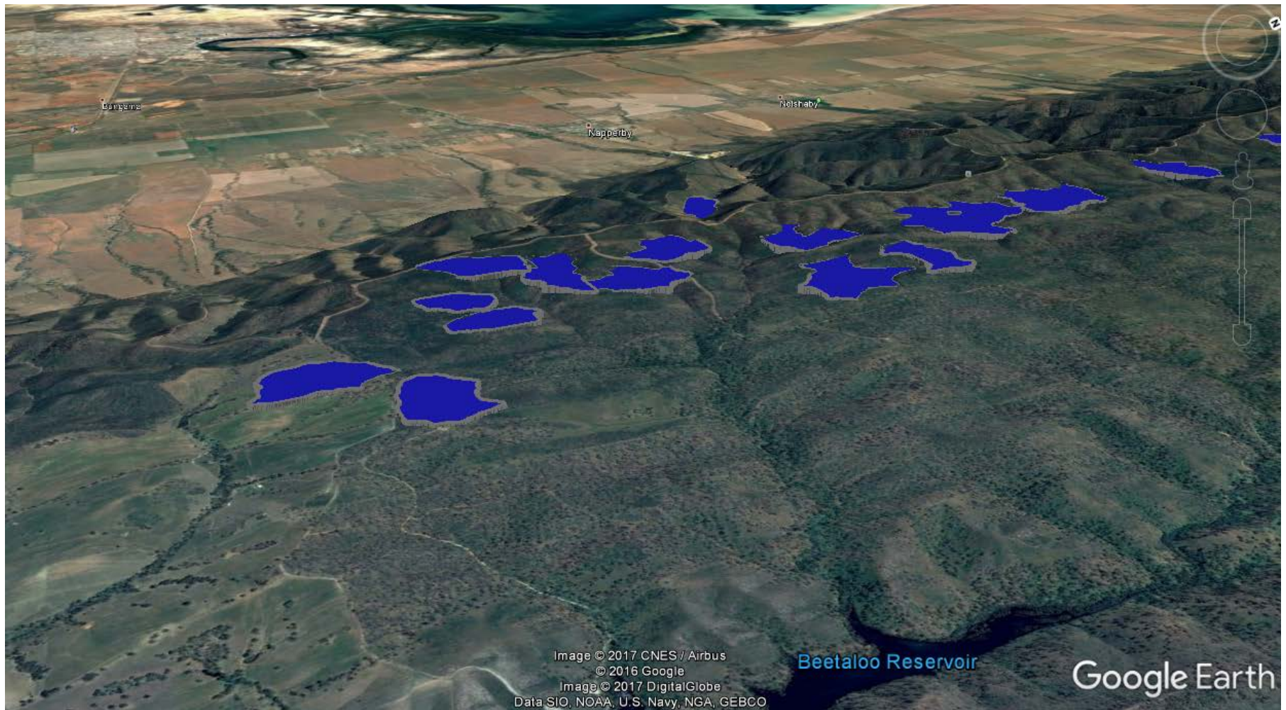
Figure 4: Potential PHES upper reservoir sites in Region C, east of Port Pirie. The lower reservoirs would be at the western foot of the hills (top of the image).
