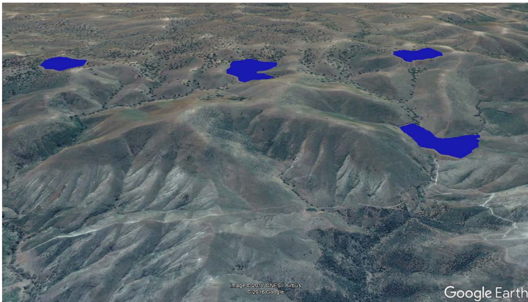
Figure 3: Potential PHES upper reservoir sites in Region B, east of Port Augusta. The lower reservoirs would be at the western foot of the hills (bottom of the image).
