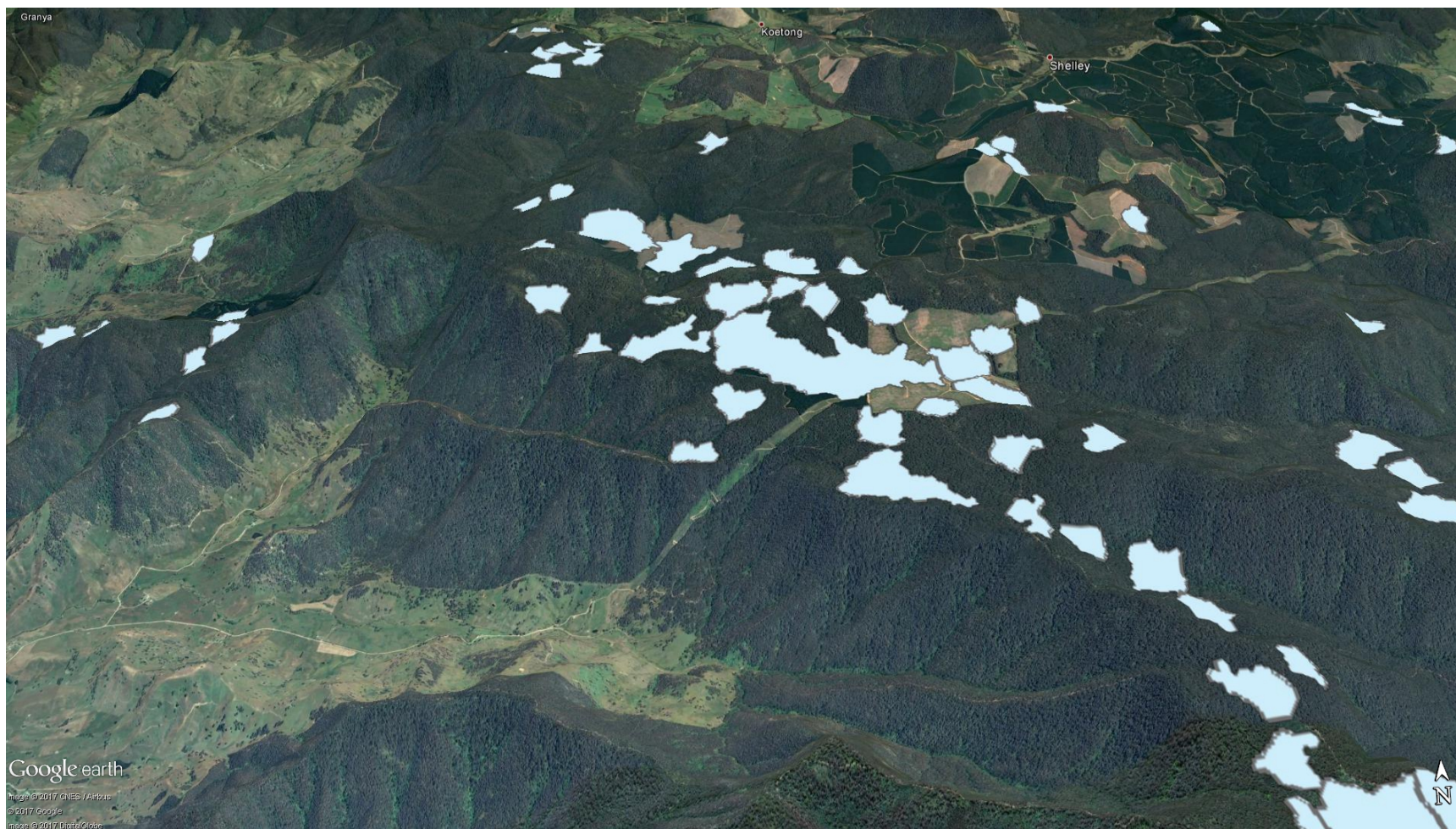
Figure 15: Potential PHES upper reservoir sites near the Tallangatta Valley (Victoria) The easement corridor for the 330 kV transmission line can be seen in this image.
