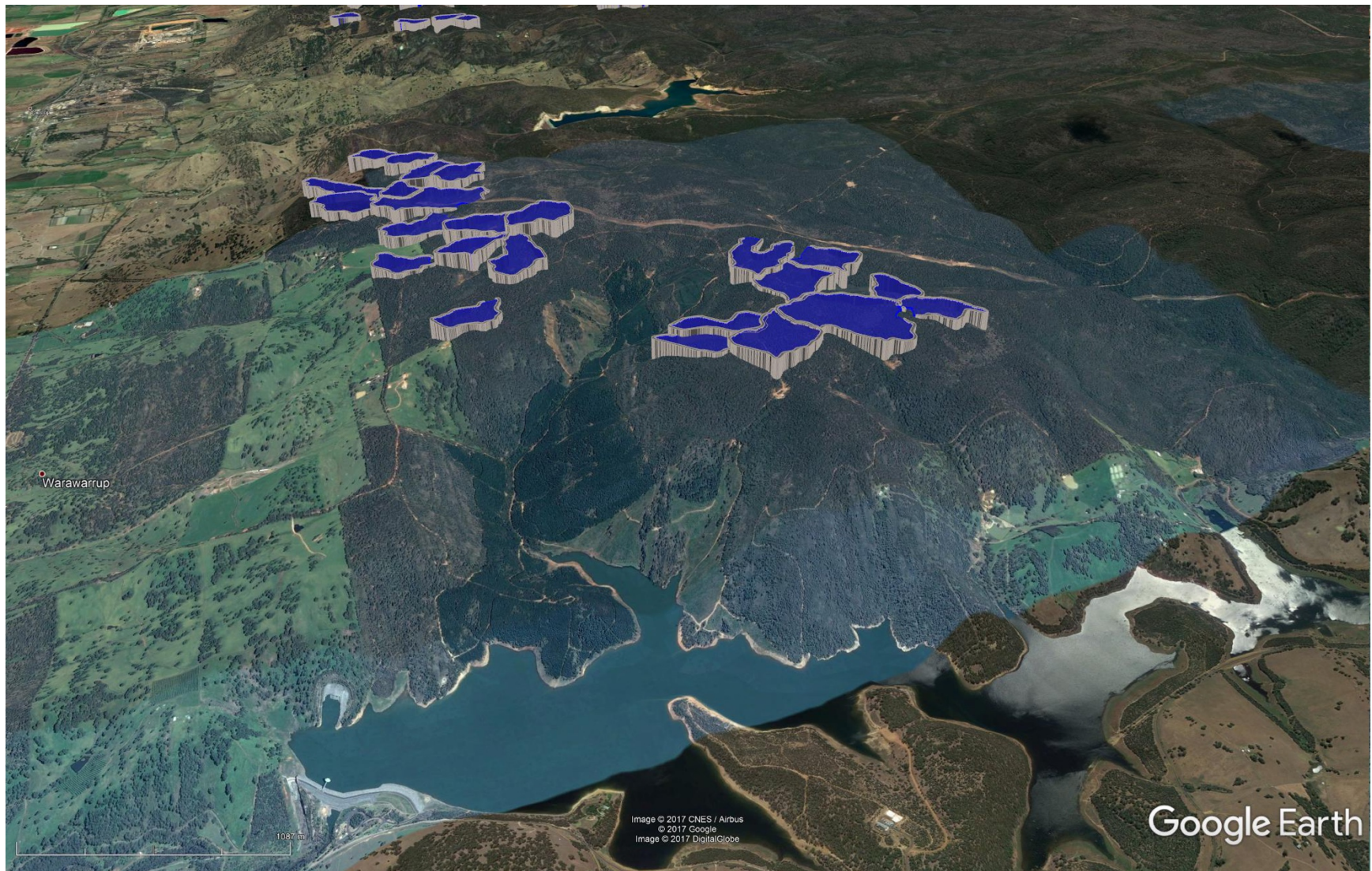
Figure 18: Potential PHES upper reservoir sites near Harvey, WA. The existing reservoir at the bottom of the image could be incorporated into a PHES system.
