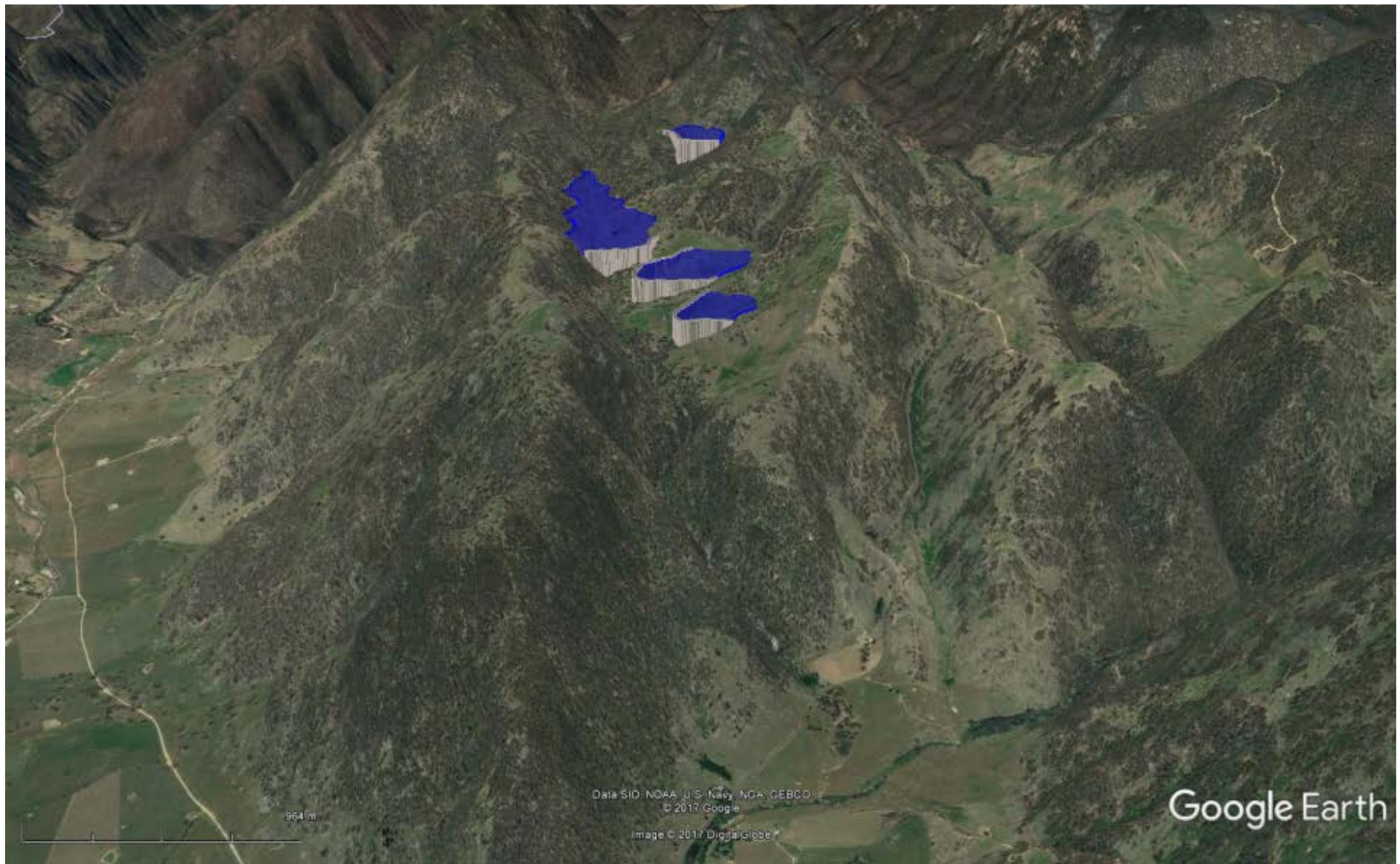
Figure 10: Potential PHES upper reservoir sites near Naas, ACT. The head is about 300 m.
