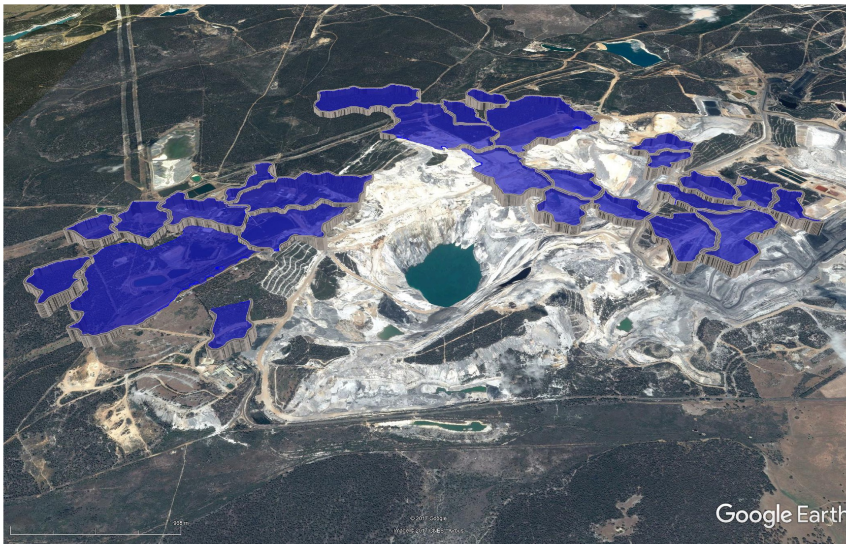
Figure 17: Potential PHES upper reservoir sites at Collie, WA, with 200 m head into the pit and a good volume of stored water.
