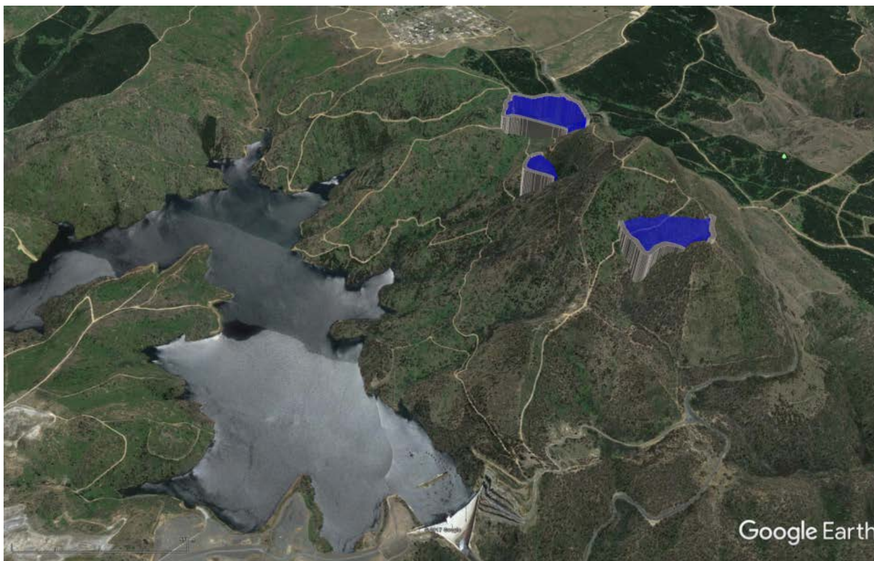
Figure 9: Potential PHES upper reservoir sites on Mt Macdonald near Cotter (ACT). The head is about 100 m rather than the 300-600 m head available elsewhere.
