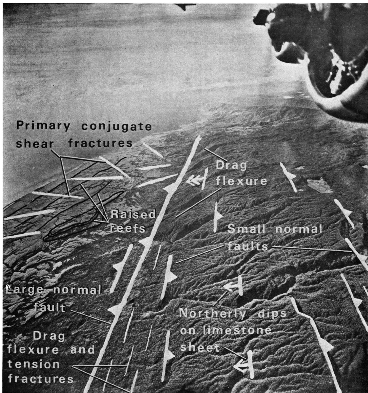
Figure 5. Oblique aerial photograph of northeastward-dipping Miocene-Pliocene limestone sheet in the Huon Peninsula, showing northward-tilted fault blocks downthrown to the south. Note the drag flexure with tension fractures of the limestone by the large normal fault at the front (north) of the sheet. Raised Quaternary coral terraces, up to 600 m high, north of the fault have been described by Chapell (1974); elements of a Holocene fracture set are evident. Note also the large bottlenecked valleys at the front of the limestone sheet cut by consequent rivers and streams. Photograph taken looking east along Huon Peninsula at about 147^{\circ} 30' E , from 8000 m.
