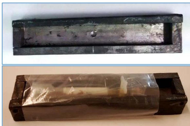
Figure H-2 Pb cradle with 6 mm diameter centre hole top view (top). A TEVA ® resin column prepared for gamma counting (bottom).
