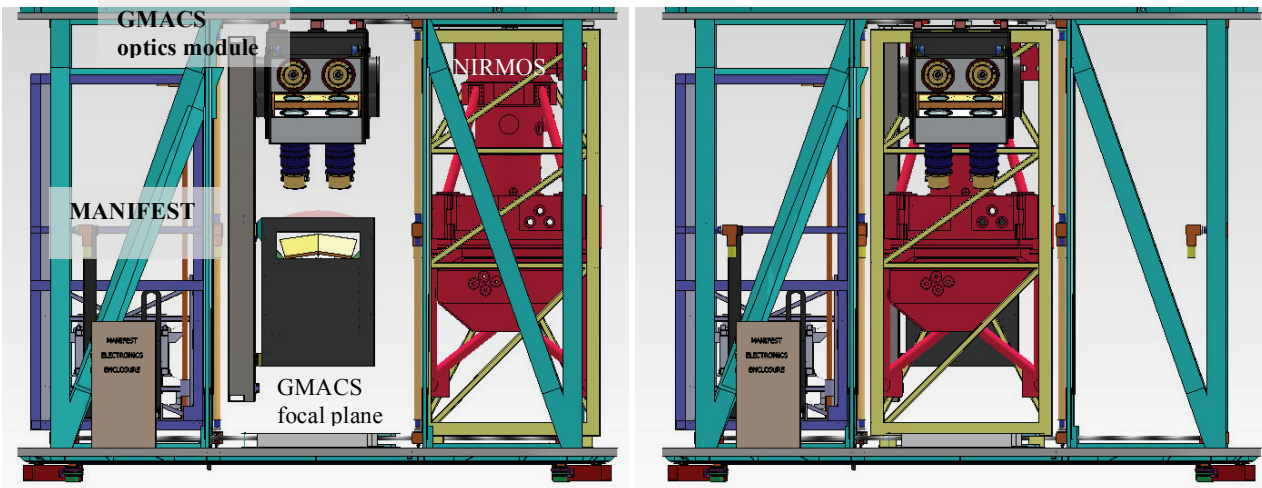
Figure 3. The GIR showing three stowed instruments (left): NIRMOS, MANIFEST, and one of the two GMACS optics modules with its optics feed (includes field lens, tent mirrors, and slit mask exchanger). The right-hand image shows NIRMOS on axis for observing.
