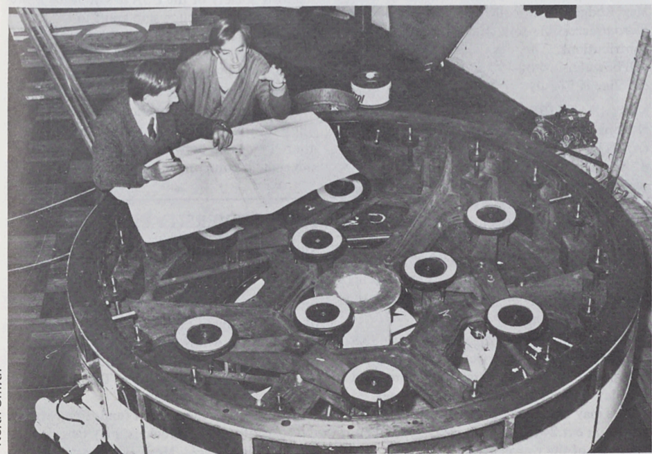
Dr Rodgers (left) and Mr Hart examining some of the mirror mountings which are supported by 36 tonnes of the moving telescope structure.
