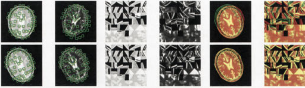
Figure 5.4: Global transformation matrix recovery test image-pairs result: The 1st row shows the situation of proton density image and T-2 weighted image initialised by affine transformation matrix 1 in table 5.2. The 2nd row presents the alignment result between them. Where 1st column contains image I_1(x) and the template \tilde{T}_1(x) ; the 2-nd column is sub-image sI_1(x) and corresponding sub-template s\tilde{T}_1(x) , which are generated with 49 15 \times 15 patches (Green squares indicate 49 patches in the in the image and the template); The 3-rd column consists of the alignment evaluation of both whole image pair ( I_1(x) and \tilde{T}_1(x) ) and sub-image pair ( sI_1(x) and s\tilde{T}_1(x) ).
