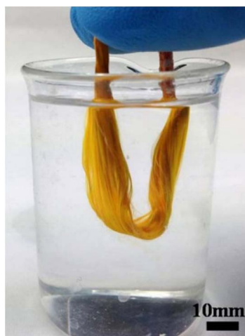
Fig. 4. Image of a FB consisting of 810,000 \text{As}_2\text{S}_3/\text{PEI} fibers after the PEI was dissolved by the DMAc solvent. The FB had a cross section of \sim 10 \text{ mm}^2 , which was obtained by further reducing the side length of the FB shown in Fig. 1(c) through the drawing process. The FB was put into a cup of water to show its flexibility more clearly.
