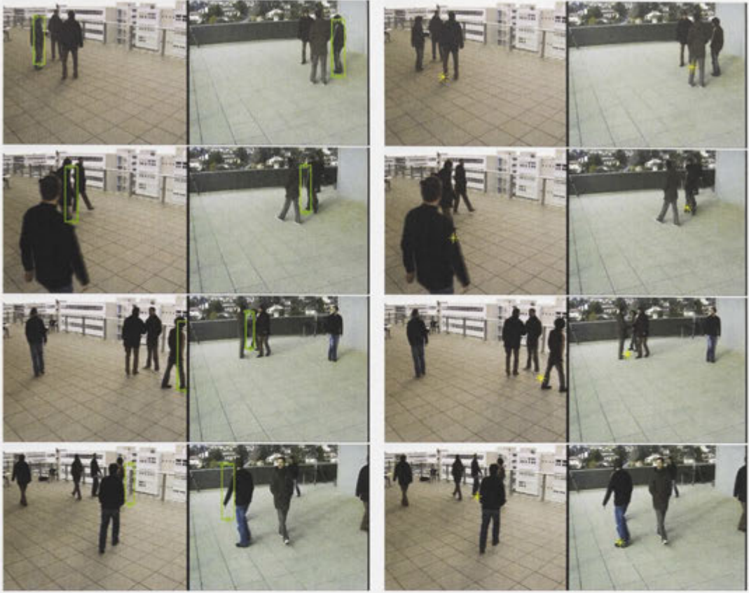
Figure 5.15: Results for the “Terrace” sequence using 2 cameras at frames 820, 875, 980 and 1143. Left: results yielded by our algorithm. Right: results yielded by the synergy map method (Khan and Shah, 2006).
