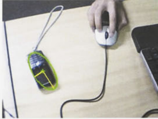
Figure 3.1: An elliptical region covering the tracking target. The orientation and size of the ellipse can be computed directly from the covariance matrix of the pixel set \mathcal{X} = \{\mathbf{x}_i\}_{i=1\dots N} .
