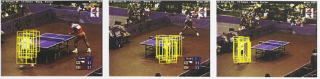
Figure 2.7: Results of the particle filter tracker proposed by Pérez et al. (2002). The yellow rectangles represent the final position of the tracking particles and the cyan rectangle is the mean position, i.e. the object position, computed as the weighted average of these particles.
