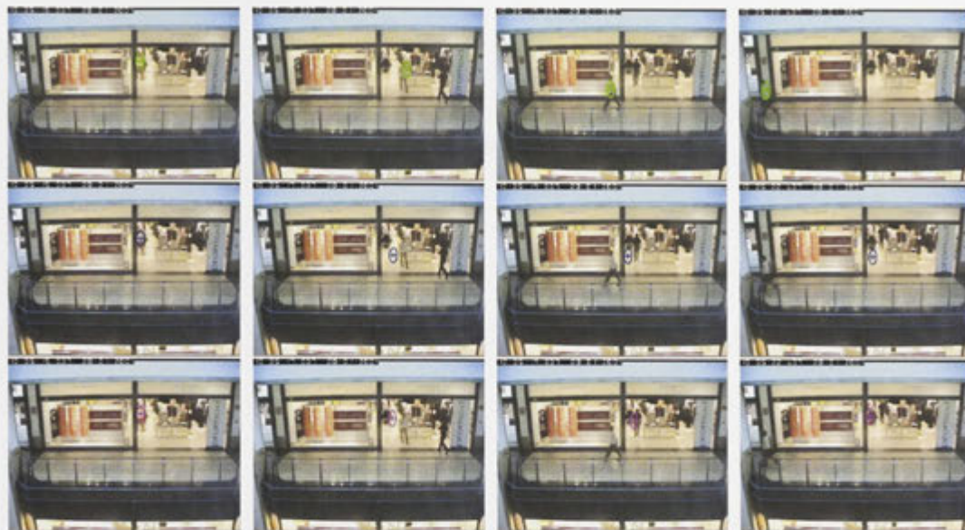
Figure 4.11: Results for the “EnterExitCrossingPath1front” sequence at frames 170, 220, 290 and 360. From top-to-bottom: results yielded by our algorithm using the 11-feature set, the on-line VR-based tracker (Collins et al., 2005) using the 11-feature set, and the on-line PCA-based tracker (Han and Davis, 2004) using the 11-feature set.
