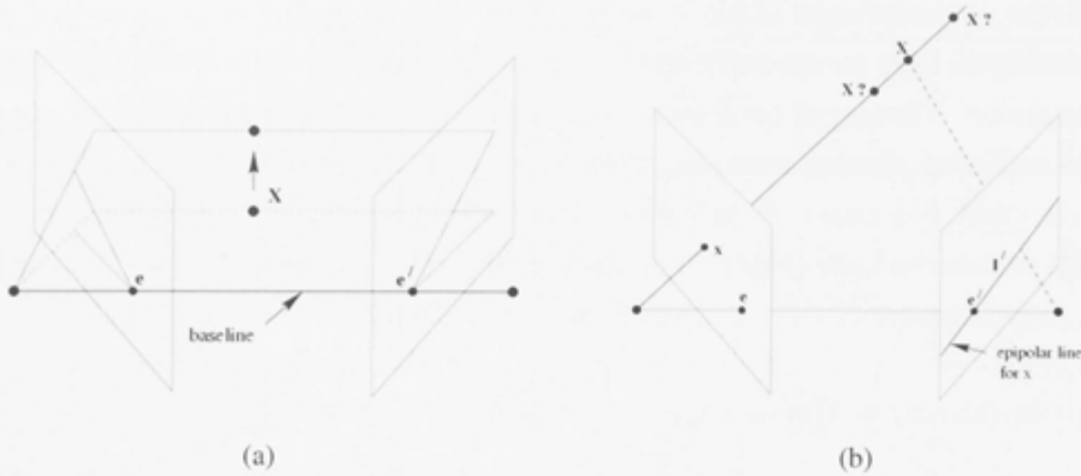
Figure 2.10: Epipolar geometry: (a) Family of planes \pi rotate around the baseline as the 3-space point X varies. (b) An image point x back-projected to a ray in 3-space defined by the first camera centre C , and x . This ray is imaged as a line l' in the second view. The 3-space point X which projects to x must lie on this ray, so the image of X in the second view must lie on l' (Hartley and Zisserman, 2004).
