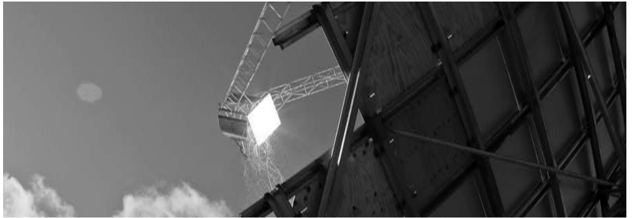
The mirrored dish concentrates the rays of the sun into a superheated point. Photos: Greg Burgess
