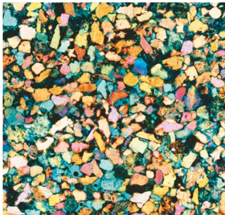
A sliver of oil-bearing rock is analysed under polarised light to show crystal placement. Image: Digital Core Lab
