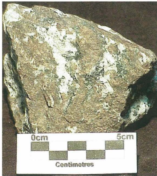
Figure 3.19 – Photo of skarned Blayney Volcanics (sample #NH59). Note predominance of garnet over wollastonite.
