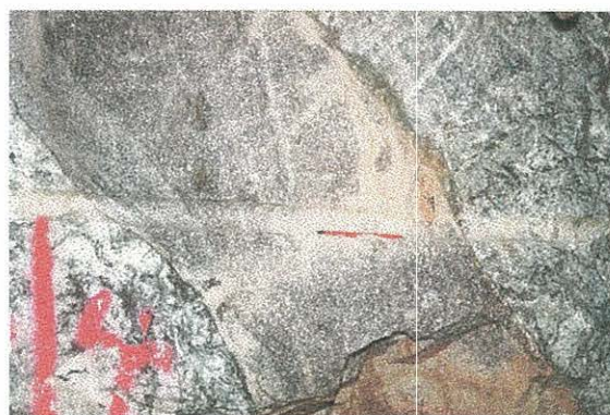
Figure 3.8 (a), (b) – Photos of two separate dykes underground with intrusive contacts (both from 10450mRL). Length of pen is 15cm.
