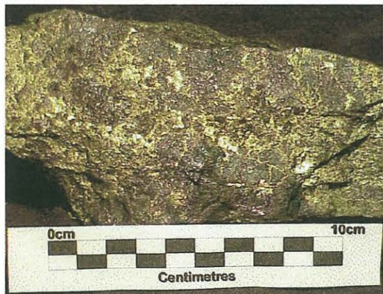
Figure 3.19 – Photo of skarned Blayney Volcanics (sample #NH59). Note predominance of garnet over wollastonite.
