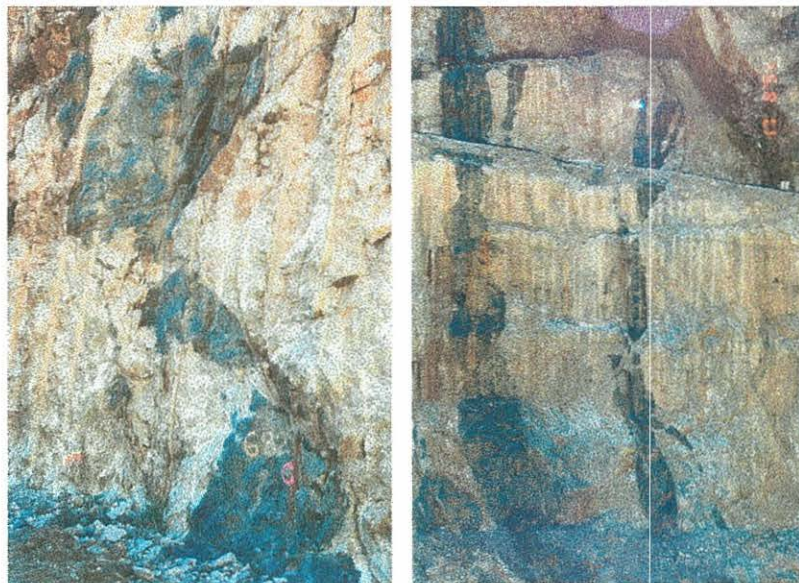
Figure 3.25 – Photos of basaltic dykes in the open pit (Rangott & Bird, 1994). Width of dykes 1-2m.
