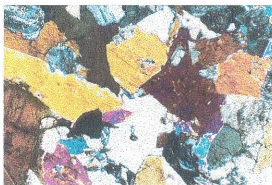
Figure 3.11 – Photomicrograph of Mine Dyke Group showing mafic silicates (sample #NH38, crossed polars, width of photo 2.45mm).
