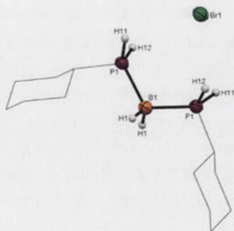
Figure 7: The molecular structure of [\text{H}_2\text{B}(\text{PH}_2\text{Cy})_2]\text{Br} . (Alkyl hydrogen atoms omitted for clarity, aryl groups simplified, 50% displacement ellipsoids). Selected bond lengths (Å) and angles ( ^\circ ): B1-P1 1.918(1); P1-B1-P1 ^i 117.0(1).
