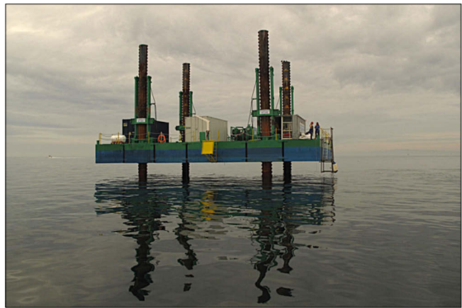
Figure 1. Jack-up Platform Barge 1—the AHSP's diving platform (Photo: A. Viduka).
