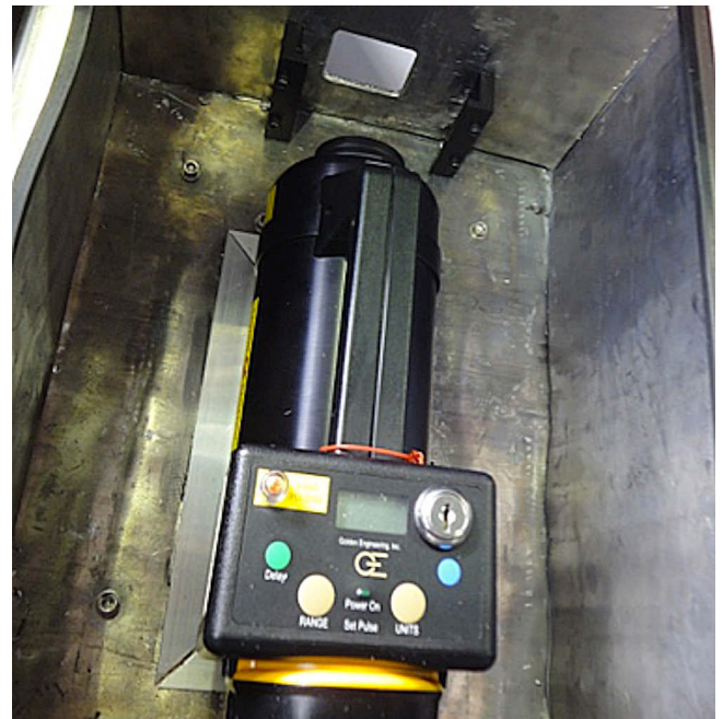
Figure 7. X-ray source in position (Photo: D. Creagh).
