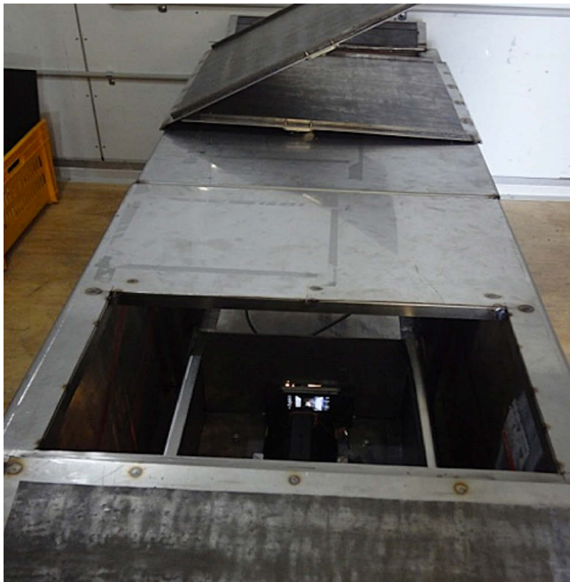
Figure 6. X-ray enclosure showing access doors for the IP, the specimen stage and the source. The photographic image on the viewing screen of the camera can be seen (Photo: D. Creagh).
