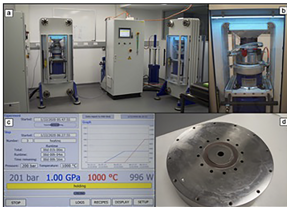
FIG. 1. The rapid quench piston cylinder apparatus at Macquarie University. (a) Laboratory with two RQPC apparatuses; (b) close-up of one RQPC apparatus with experiment running; (c) control panel with touch-screen programmable ramps for temperature and pressure; (d) Strecon pressure vessel with additional cooling channels close to the tungsten carbide core, which improve cooling rate and core lifetime.
