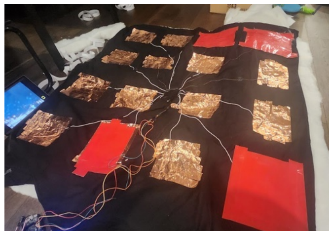
Figure 3.16: Expanded copper tape pads (16 September 2024)
